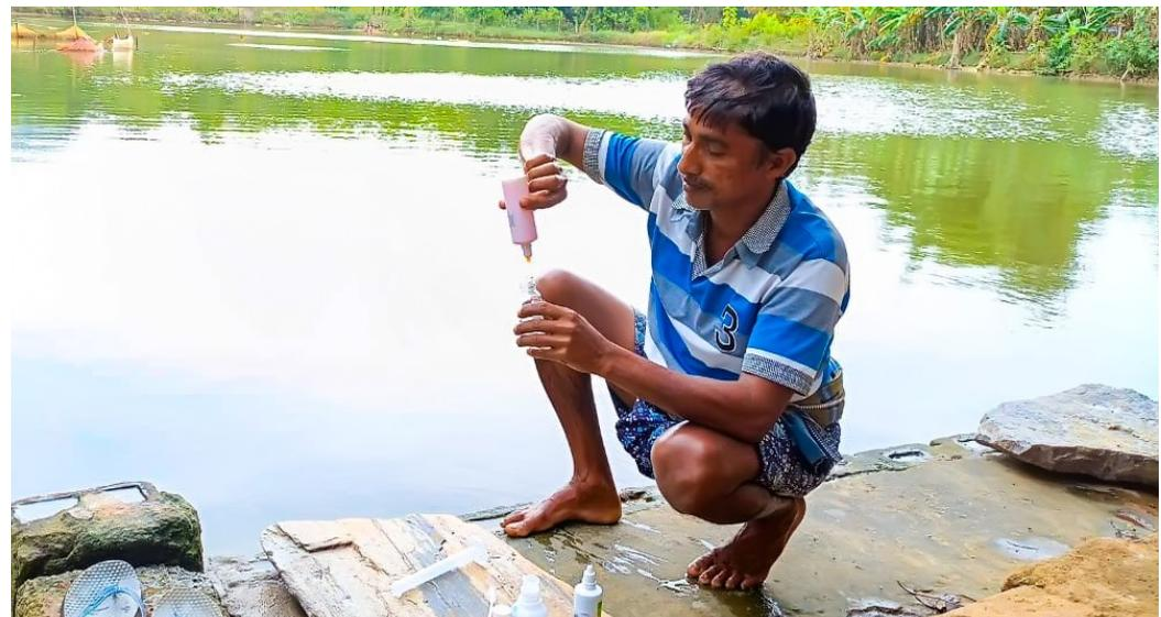
Water testing kit to monitor water quality parameters for adaptive measures to increase fish production in this climate changing scenario
